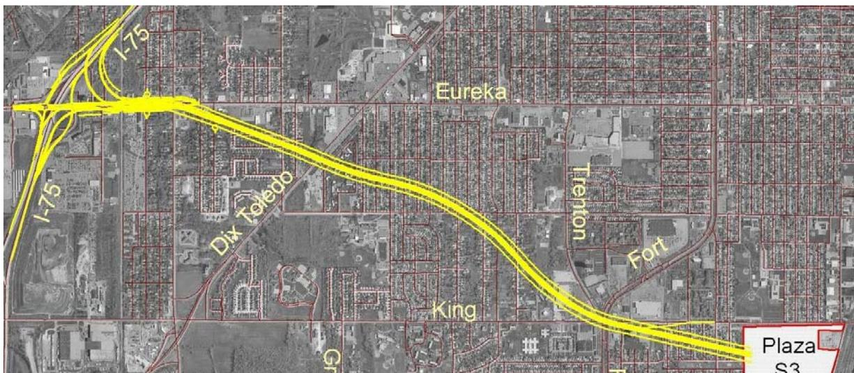
**Segment B:** This potential alignment is approximately 7.80 miles long and is primarily on the south side of Eureka Road. The alignment intersects residential area with some retail and commercial uses. This potential route will require the reconstruction of the I-75 and Eureka interchange and also the construction of an interchange at Eureka and the Airport Road.
