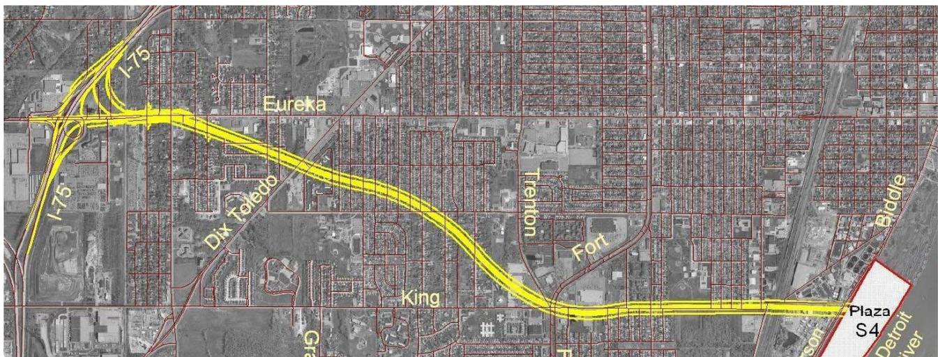
**Segment B:** This potential alignment is approximately 7.80 miles long and travels on the south side of Eureka Road. The alignment intersects primarily residential area with some retail, commercial and a school. This potential route will require the reconstruction of the I-75 and Eureka interchange and also the construction of an interchange at Eureka and the Airport Road.
