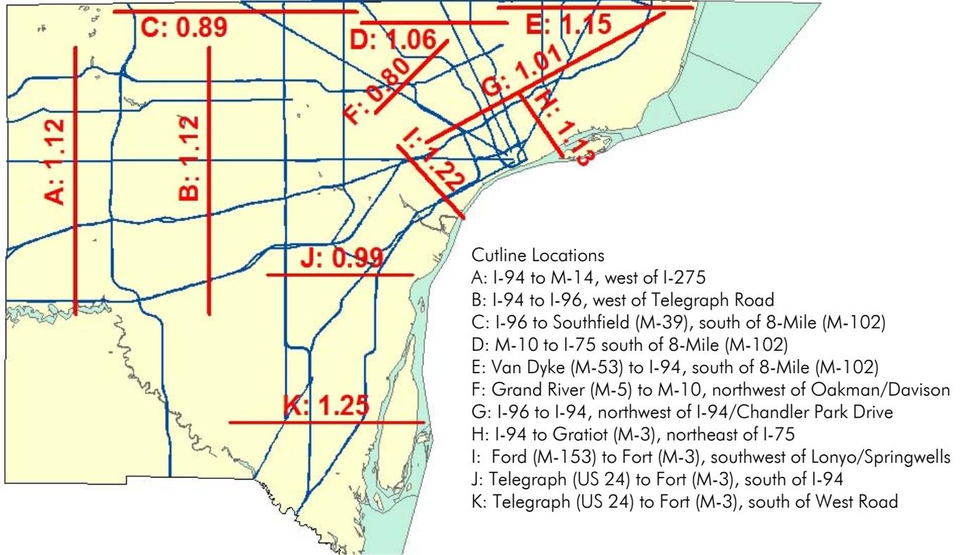
Note: The values labeled in each cutline are the ratio of MDOT 2004 Sufficiency File AADT to model traffic volume.
