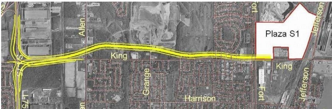
**Segment B:** The potential alignment is approximately 7.80 miles long aligned with the existing King Road from I-75 to Vining Road before it bends diagonally to the interchange at I-275 and Sibley Road. The alignment intersects commercial development, residential uses and undeveloped land. This potential alignment will require a new fully directional interchange at I-75 and King Road and also reconstruction of the interchange at I-275 and Sibley Road.
