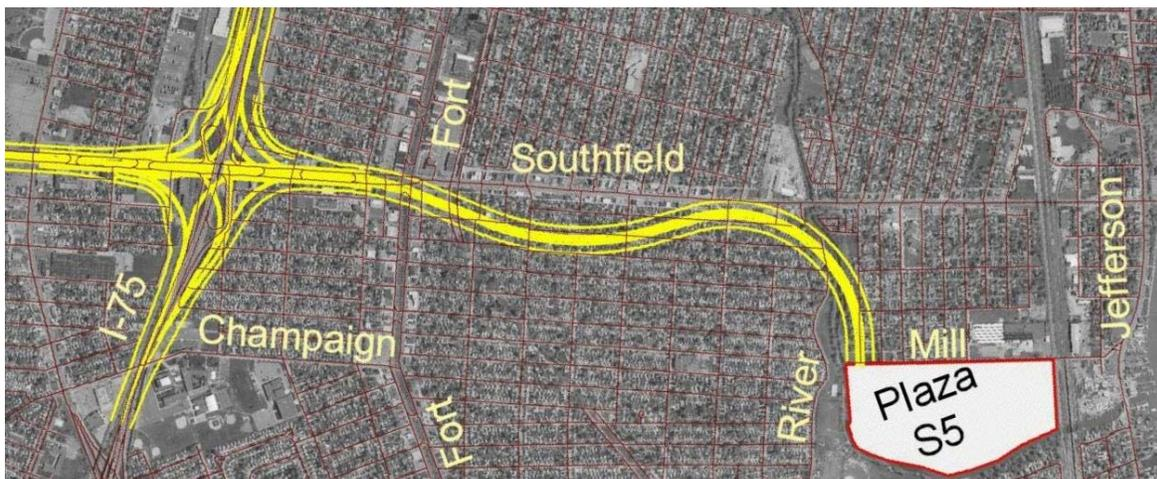
**Segment B:** This potential alignment would convert Southfield Highway to a limited access facility between I-75 and the I-94 interchange.
