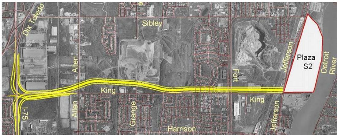
**Segment B:** The potential alignment is approximately 7.80 miles long aligned with the existing King Road from I-75 to Vining Road before it bends diagonally to the interchange at I-275 and Sibley Road. The alignment intersects commercial development, residential uses and undeveloped land. This potential alignment will require a new fully directional interchange at I-75 and King Road and also reconstruction of the interchange at I-275 and Sibley Road.
